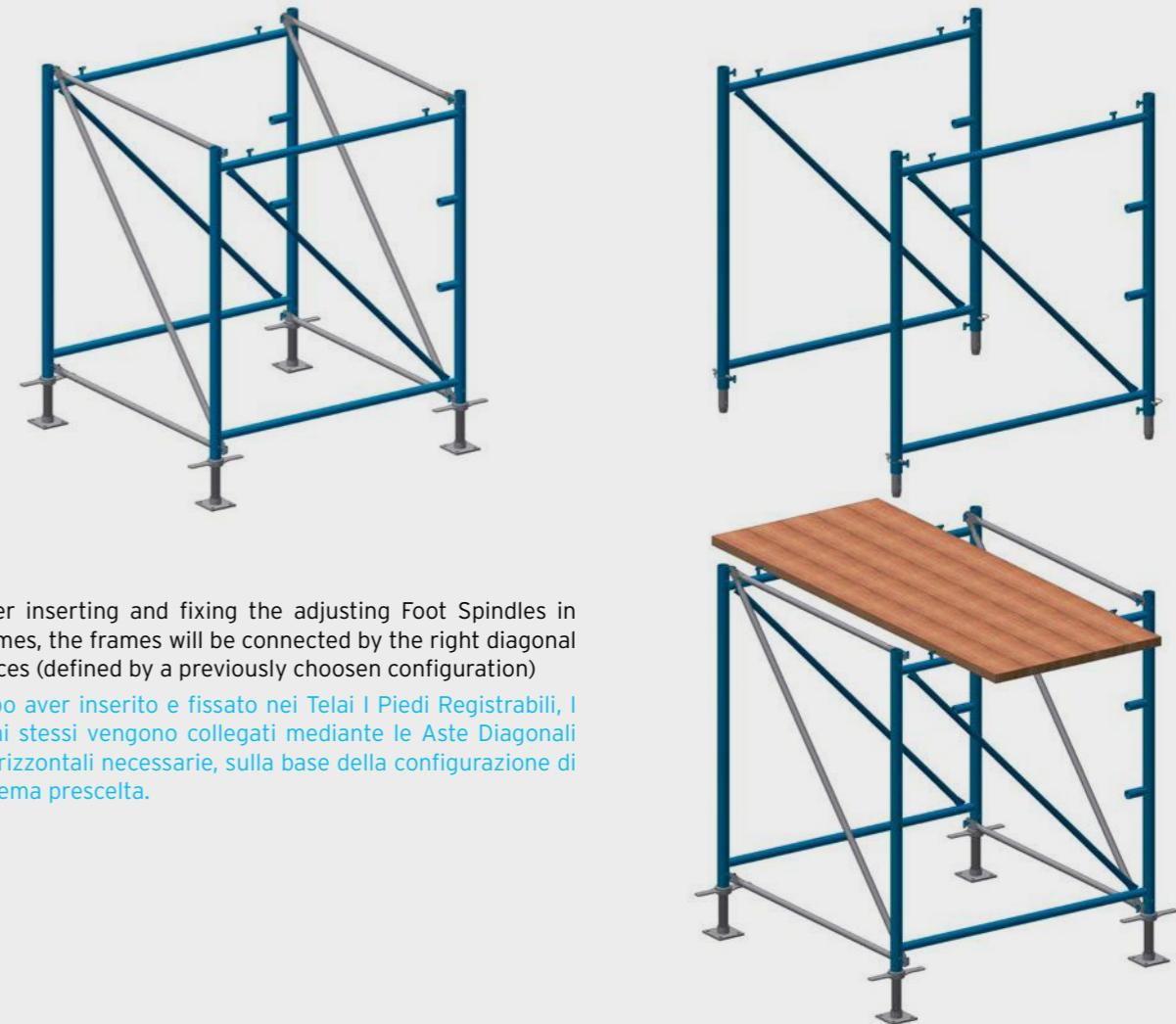
After inserting and fixing the adjusting Foot Spindles in Frames, the frames will be connected by the right diagonal braces (defined by a previously chosen configuration)
