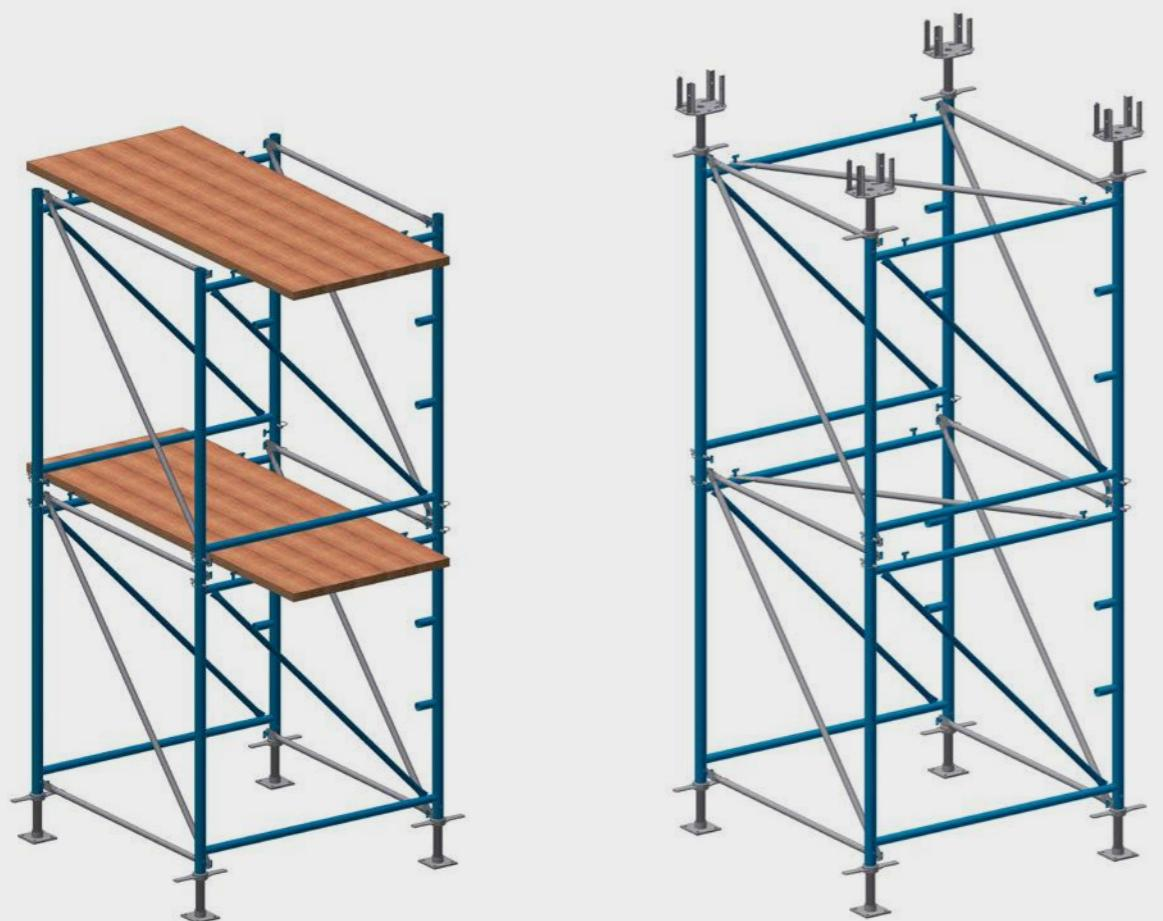
Always to ensure a proper tower anchorage to the ground or near structures in order to guarantee the necessary stability during the assembling, other than provide any necessary safety device as safety harness for all working staff members
