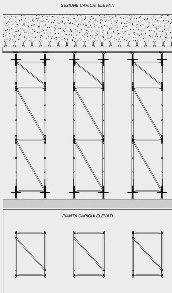
When slabs loads become relevant, the span between towers legs have to be reduced, and that's easily done by combining the right system components (shorter horizontal and diagonal braces).
