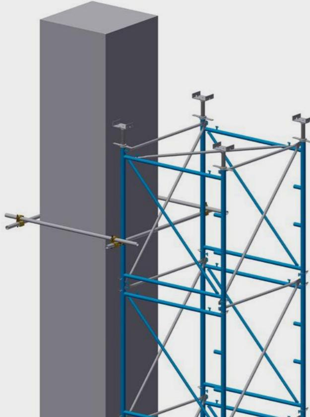
Max distance between anchoring plans 8 m
