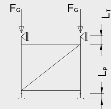
! To maximize the load capacity on the leg, set the extractions of the head less than that of the foot.
