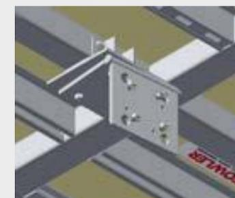
To be used for props connection to lateral 1800 formwork elements, in wing configuration, and in combination with "Prop bracket-wing panel". It can be fixed to formworks panels by bolts or pins.
